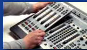
Module installation and removal couldn't be simpler. Single Ethernet cable connects modules to frame.
