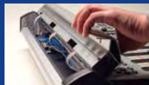
Hinged bridge gives easy access to Element's connection panel. One-cable connection to power, CPU.
